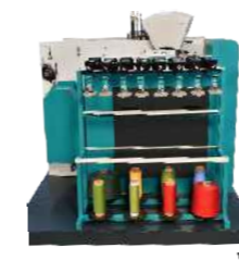
Integrated Stationary Creel
