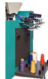
Integrated Stationary Creel
