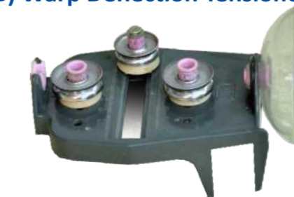
This system is used for adjustment of tension suitable for a wide range of yarns.
